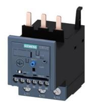
Overload relay 20...80 A Electronic For motor protection Size S2, Class 10E Contactor mounting Main circuit: Screw Auxiliary circuit: Screw Manual-Automatic-Reset
