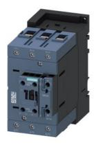
power contactor, AC-3 110 A, 55 kW / 400 V, 1 NO + 1 NC, 230 V AC, 50 Hz 3-pole, 3NO, Size S3 screw terminal
