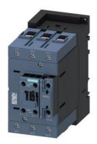
power contactor, AC-3, 110 A 1 NO + 1 NC, 20-33 V AC/DC 3-pole, 3NO, size S3 screw terminal varistor integrated varistor
