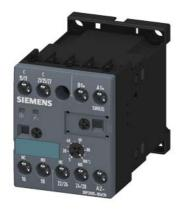
Timing relay, electronic Multifunction, 16 functions 2 change-over contacts 24 to 240 V AC/DC at 50/60 Hz AC 0.05 s to 100 h Overall width 45 mm screw terminal
