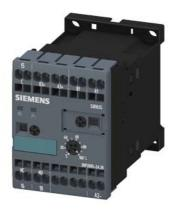
Timing relay, electronic Multifunction, 8 functions 1 change-over contact 24 V AC/DC, 100 AC to 127 V at 50/60 Hz AC 0.05 s to 100 h Overall width 45 mm Spring-type terminal
