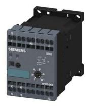
Timing relay, electronic ansprechverzögert 1 change-over contact 24 V AC/DC, 200 to 240 V AC at 50/60 Hz AC 0.05 s to 100 h Overall width 45 mm Spring-type terminal
