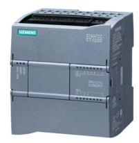
SIMATIC S7-1200, CPU 1211C, compact CPU, AC/DC/relay, onboard I/O: 6 DI 24 V DC; 4 DO relay 2A; 2 AI 0-10 V DC, Power supply: AC 85-264 V AC at 47-63 Hz, Program/data memory 50 KB
