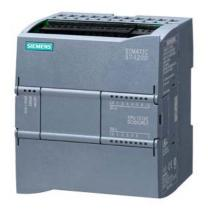
SIMATIC S7-1200, CPU 1212C, compact CPU, DC/DC/relay, onboard I/O: 8 DI 24 V DC; 6 DO relay 2 A; 2 AI 0-10 V DC, Power supply: DC 20.4-28.8V DC, Program/data memory 75 KB
