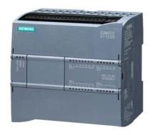
SIMATIC S7-1200, CPU 1214C, compact CPU, AC/DC/relay, onboard I/O: 14 DI 24 V DC; 10 DO relay 2 A; 2 AI 0-10 V DC, Power supply: AC 85-264 V AC at 47-63 Hz, Program/data memory 100 KB
