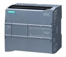
SIMATIC S7-1200, CPU 1214C, compact CPU, DC/DC/relay, onboard I/O: 14 DI 24 V DC; 10 DO relay 2 A; 2 AI 0-10 V DC, power supply: DC 20.4-28.8 V DC, program/data memory 100 KB
