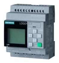
\*\*\*spare part\*\*\* SIPLUS LOGO! 24RCE based on 6ED1052-1HB08-0BA0 with conformal coating, -25...+60 °C, start up -20 °C, logic module,display power supply / I/O: 24 V AC/24 V DC/relay, 8 DI/4 DQ, memory 400 blocks, modularly expandable, Ethernet, integrated web server, data log, user-defined web pages, standard microSD card for LOGO! Soft Comfort V8 or higher, older projects executable
