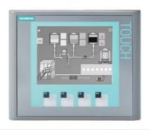
\*\*\*spare part\*\*\* SIPLUS HMI KTP400 Basic mono PN based on 6AV6647-0AA11-3AX0 with conformal coating, -10...+60  $^{\circ}$ C, display, Ethernet interface
