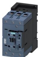
power contactor, AC-3e/AC-3, 110 A, 55 kW / 400 V, 3-pole, 20-33 V AC/DC, with integrated varistor, auxiliary contacts: 1 NO + 1 NC, screw terminal
