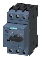
Circuit breaker size S00 for motor protection, CLASS 10 A-release 0.45...0.63 A N-release 8.2 A screw terminal Standard switching capacity
