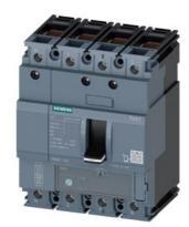
circuit breaker 3VA1 IEC frame 160 breaking capacity class S Icu=36kA @ 415V 4-pole, line protection TM220, ATFM, In=100A overload protection Ir=70A...100A short-circuit protection Ii=10 x In N conductor unprotected clamp connection
