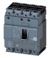
circuit breaker 3VA1 IEC frame 160 breaking capacity class S Icu=36kA @ 415V 4-pole, line protection TM220, ATFM, In=160A overload protection Ir=112A...160A short-circuit protection Ii=10 x In N conductor unprotected clamp connection
