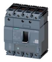
circuit breaker 3VA1 IEC frame 160 breaking capacity class S Icu=36kA @ 415V 4-pole, line protection TM220, ATFM, In=40A overload protection Ir=28A...40A short-circuit protection Ii=10 x In N conductor unprotected clamp connection
