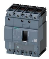
circuit breaker 3VA1 IEC frame 160 breaking capacity class S Icu=36kA @ 415V 4-pole, line protection TM220, ATFM, In=16A overload protection Ir=11A...16A short-circuit protection Ii=20 x In N conductor unprotected clamp connection
