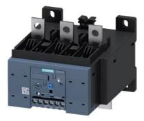
Overload relay 50...200 A for motor protection Size S6, Class 10E Contactor mounting/stand-alone installation Main circuit: busbar connection Auxiliary circuit: Screw terminal Manual-Automatic-Reset
