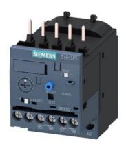
Overload relay 0.32...1.25 A Electronic For motor protection Size S00, Class 10E Contactor mounting Main circuit: Screw Auxiliary circuit: Screw Manual-Automatic-Reset
