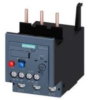
Overload relay 47...57 A Thermal For motor protection Size S2, Class 10 Contactor mounting Main circuit: Screw Auxiliary circuit: Screw Manual-Automatic-Reset
