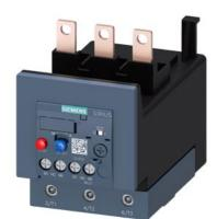
Overload relay 57...75 A Thermal For motor protection Size S3, Class 10 Contactor mounting Main circuit: Screw Auxiliary circuit: Screw Manual-Automatic-Reset
